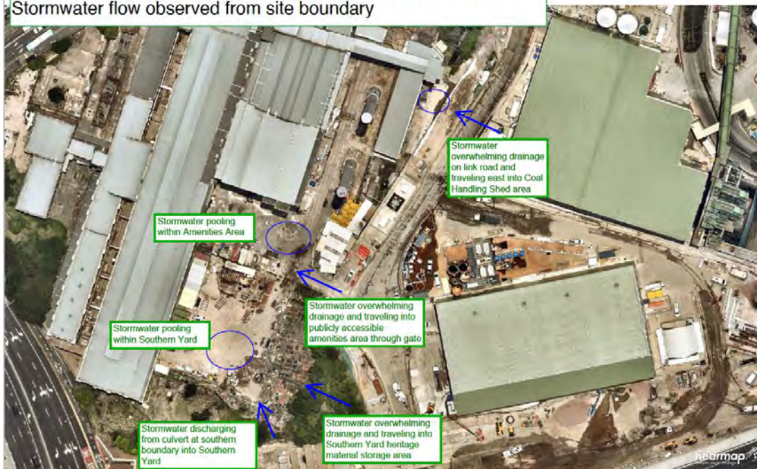
Figure 22: Observed stormwater inundation points during weather events (Nearmap modified by CBRE)
